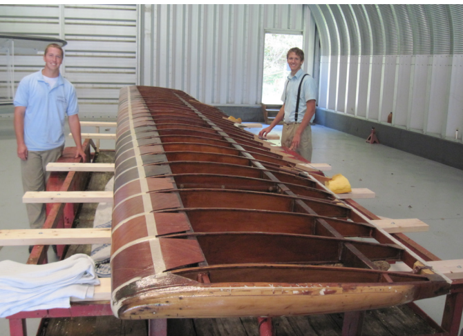
Cliff Daly (right) and his brother Joe take delivery of the one-piece Fokker D.VII upper wing.
